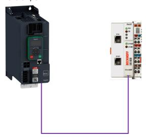
The drive is controlled from the fieldbus (EtherCAT) but the reference value is adjusted with analog input 1. The control word comes from the controller and is written according to CiA 402 profile.
