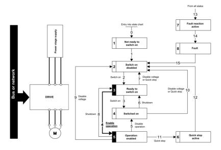
**NOTE:** It is possible, but not necessary to apply the 3 - Switch on command followed by the 4 - Enable Operation command to switch successively into the operating states 3 - Ready to Switch on, 4 - Switched on and then 5 - Operation Enabled. The 4 - Enable operation command is sufficient.
